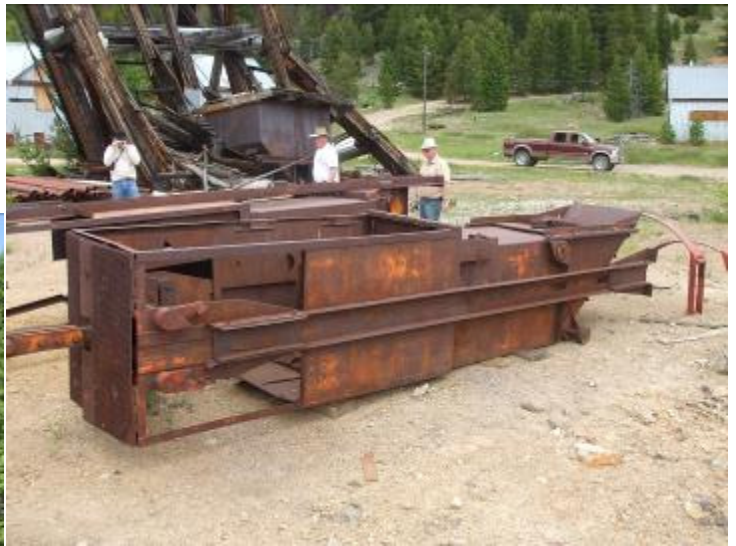
Dick Lenzer, Harold Huber & Kermit Zeiler looking at a Combination Skip. (Men on top and Ore on bottom) By-Metallic Mine in Granite, MT
